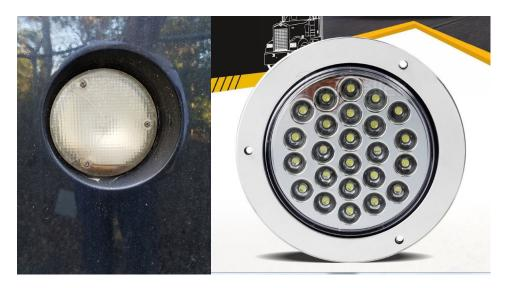
The lenses provided by Fleetwood are 5" across but I have been unable to locate an LED lens with the three screw configuration at that size. Those with three mounting screws appear as 4" lenses but the mounting rings are more than 5" in diameter. In the example above, the mounting ring is 6" in diameter.
