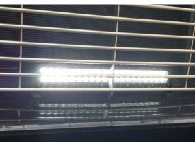
The backup lights come on when the coach is in reverse, just as before. But now, if I need more light to back into a dark storage location, I can flood the area with light by turning on the Light Bar along with the Docking Lights at the driver's seat.
