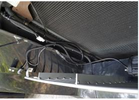
The light bar is between the radiator and the rear grill. The manual light switch is between the lower grill and the upper grill (open). The main wiring to the battery compartment exits at the top left of the radiator.
