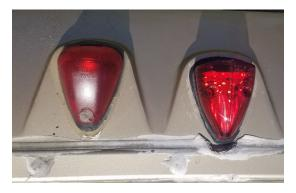
We soon discovered a problem. Clearance Lights should flash with the ICC switch at the driver's seat. If the clearance lights are ON, they should flash OFF. If they are OFF, they should flash ON so that they can send a 'Thank You' to other drivers day or night. Well, after replacing the original incandescent lights with LED lights they will flash OFF OK if the lights are ON but NOT the other way around.
