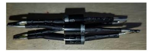
**Parts:** Butt Connectors from Amazon (smaller quantities are available at Lowes or Home Depot). Use a crimping tool to ensure tight connections.
