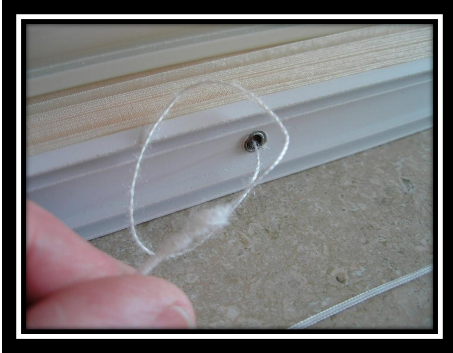
Picture 1 – The eyelet shown is the crimped over part of a 1-piece eyelet installed by the manufacturer. The cord after passing through the top has to pass over this rough part of the eyelet with considerable tension. In every set of blinds with frayed cords this will be found.
