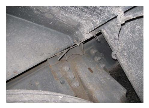
3. Passenger Side rear wheel well bracket aft of the axle is broken
