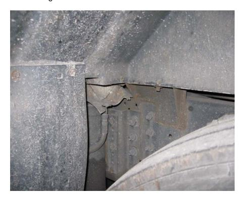
4. Passenger side bracket forward of the axle is cracked (the bright colored spot) and the bolt is bent
