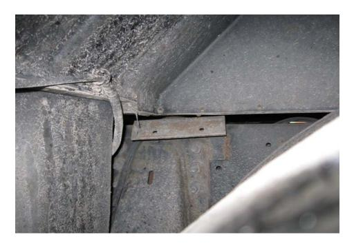
2. Driver Side rear wheel well the bracket aft of the axle is broken
