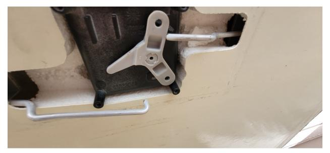
Step 2: Remove the square drive screws from the latch mechanism(some latches are riveted, and some may have a hidden nut in the door, and improvedryparts.com has a great instruction set for those who may need it.)
