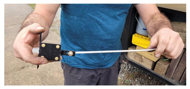
Step 8: Slide the latch mechanism back in place. If it need extra effort to seat the latch, make sure that it is assembled tightly. I had a few that had to be tapped into place with a mallet and block.
