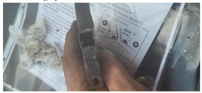
Step 4: Using a 5/32" bit (and I do recommend a drill press if available) drill out each of the four rivets. The rivets are usually brass or aluminum. Be careful not to let the spring get away from you when you pop off the last rivet.
