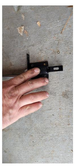
Step 6: Put the latch assembly together and put on top of a rivet (use a hard surface such as a metal table or in my case I used the shop floor.) Then while holding the assembly together tightly, place the rivet tool over the rivet and hit it with a hammer. Repeat with all four rivets and inspect the assembly to ensure that it is snug and no rivets are loose.
