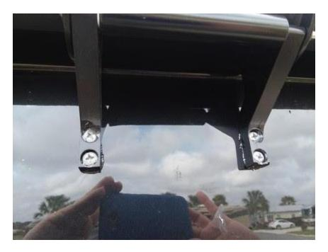
Now it is time to install the two 7/16 bolts and Nylock nuts through the arms and holes in the frame to lock the upper roller in position. Easy but having a 7/16" ratchet wrench and a 7/16" box end is helpful but not required. You can also see that the excess Goop has been wiped off.
