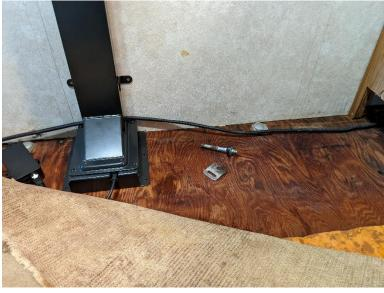
The TV Mount base (I ground off the tops of the seat belt bolts as my cabinets would have solid bottoms). Manage sparks while doing so to avoid a fire.
