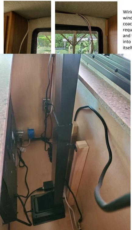
Wiring bundles in the wireway above the window - this wireway runs the length of the coach from what I could tell. Accessing it required removal of the passenger side speaker and the ceiling fabric covered pieces that screw into the ceiling to cover it. The window valence itself covers the portion above the window.
