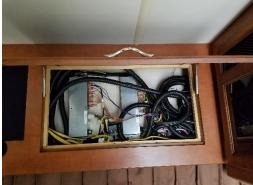
• A/C Power Line - we opened the cover on the Precision Control Power Panel and located the 3<sup>rd</sup> A/C power line as well as the open slot for the new circuit breaker.
