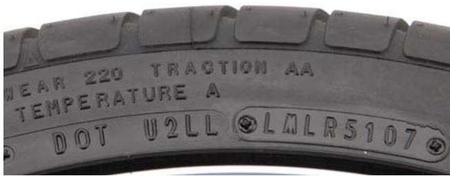
Figure 1 – Example of a tire manufactured since 2000 with the current tire identification number format. This tire was manufactured in the 51st week of 2007.
