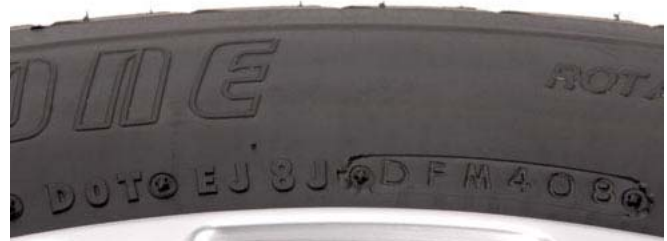
Figure 3 – This tire was manufactured in the 40th week of the 8th year of the decade ... but which decade?
