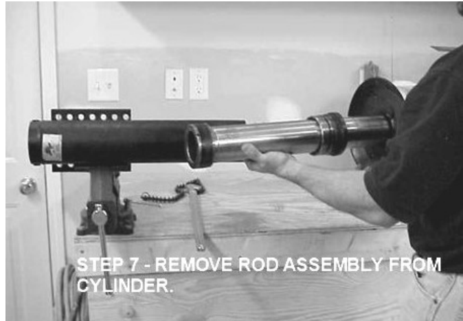
An example of the clear illustrations in the Power Gear information document Rod and Pauline used as a guide to repair the D's leaking jacks
